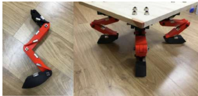
[Fig. 11] Complete model (left: leg, right: full skeleton structure)
